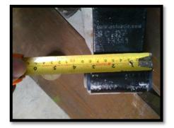
The Sulastic shackle models: SA-07, SA-07 HD, SC-07, SC-07 HD; have a width 3 ½" (3 3/8" sulastic bushing with a 1/8" washer installed in the frame side), which is the size that almost all Dodge stock shackles have.
