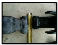
Determine if your truck has a stock shackle of 4" or  $4\frac{1}{2}$ ". If so, ask for the  $\frac{1}{2}$ " steel separator that is installed in the frame side, Two steel separators are needed for 4" and four steel separators for  $4\frac{1}{2}$ " width.
