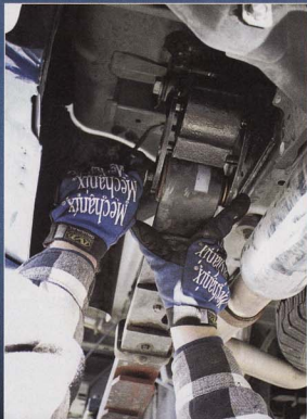
To install the Sulastic rubber springs, simply reverse the removal order of the stock shackle hangers. Washer shims are provided to ensure a proper fit of the shackle to the leaf spring and frame of the truck.
