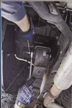
Installation on the Dodge was straightforward. After securing the axle and the frame of the truck, the shackle bolts were removed.
