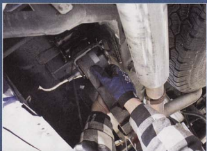
The leaf spring was pulled down to remove the lower bolt, which attaches the leaf spring to the rear shackle mount.
