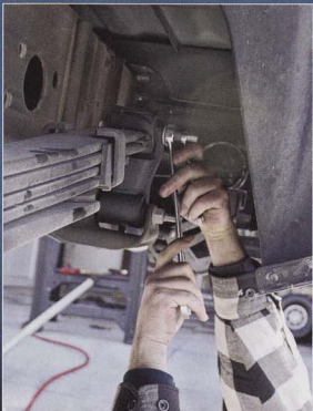
Installation on the Chevy required the same basic steps as the Dodge, except the receiver hitch was removed so that we could remove the lower shackle bolt.
