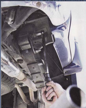
The final step is to ensure the shackle bolts are tightened to the correct torque specifications.
