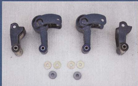
Here is a side-by-side comparison of the Sulastic rubber springs (inside) next to the OEM stock shackle hangers.
