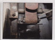
We decided to install the bolts opposite from how they came from the factory. We reasoned that since we cut the excess bolt length off, they were the same size as the nut ends and wouldn't rub.
