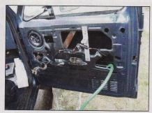
The 6½-inch Pioneer speakers fit nicely in the door in the original screw holes. We removed the dusty insulation and carefully hosed down the inside of the doors. We used heat-shrink crimp connectors and electrical tape on all the electrical connections.
