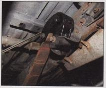
The Sulastic springs do not affect the ride height but are supposed to help with braking, cornering, and carrying heavy loads. So far, we are very impressed with the smooth difference we got from the Sulastic springs.
