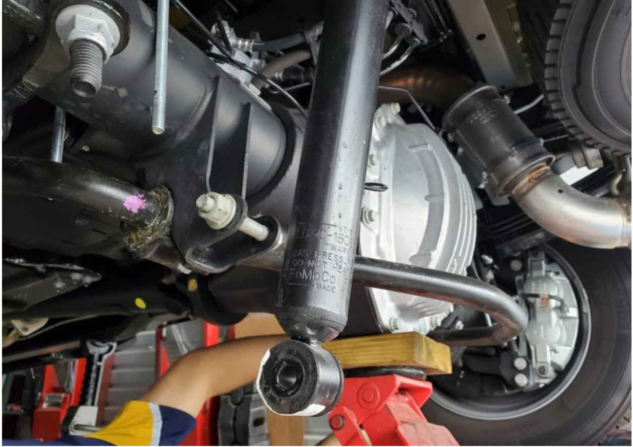
Shock absorbers removed from the bottom bolt.
