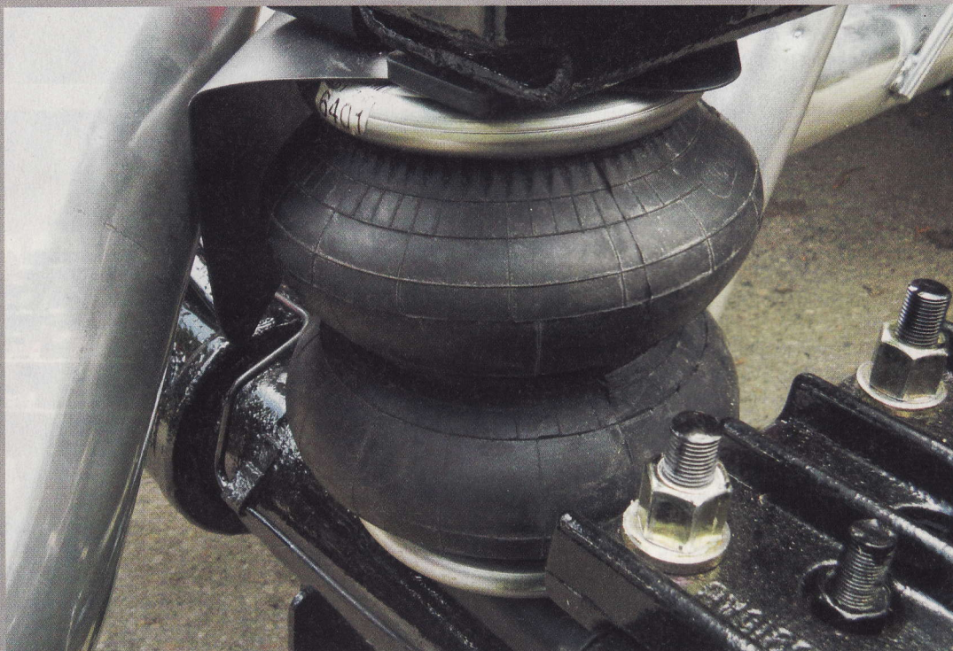
Ride-Rite air helper springs install without welding.
