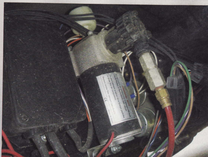
(Above) Sulastic Rubber Spring replaces factory shackle. (Below) Air pump and wireless controls mount on frame rail.
